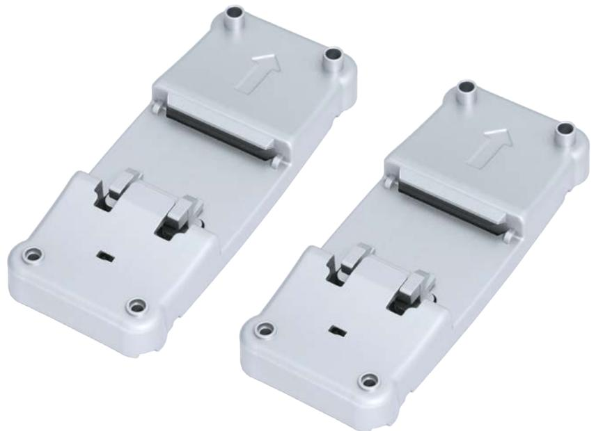
Victoria, BC, Canada – The MP-DINRAIL is a two piece ABS adapter that is custom designed to convert the standard MACH-ProCom, MACH-ProSys, MACH-ProPoint, and MACH-Pro1/2 enclosures to be DIN rail mountable. Adapter kits use the standard #8 TEK screws that ship with the controllers to fasten the adapter to the enclosure.
