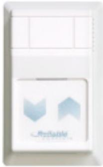
The latest addition to the Reliable Controls® product line is a two wire room temperature sensor that features setpoint adjust. Temperature is monitored by a 10k thermistor that connects to a standard Reliable Controls® 10k pullup Input point. Setpoint adjust is accomplished through Control-BASIC™ code that reacts to presses on the tactile buttons behind the intuitive Up/Down chevrons on the product face.
