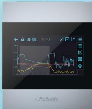
*TRENDview: Allows users easy access to their trended system data, either Single-point or Multipoint Trend Logs, without the need for a PC or any other external device.*
