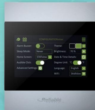
*CONFIGURATIONview: An interface to view and modify the MACH-ProView LCD user interface settings, Wi-Fi settings, and advanced connection settings. Adjust default display options such as language and LCD brightness.*
