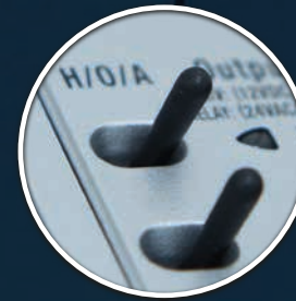
H/O/A switches with software feedback
