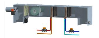
Modulate cooling and heating simultaneously to control humidity while maintaining supply air temperature at setpoint.
