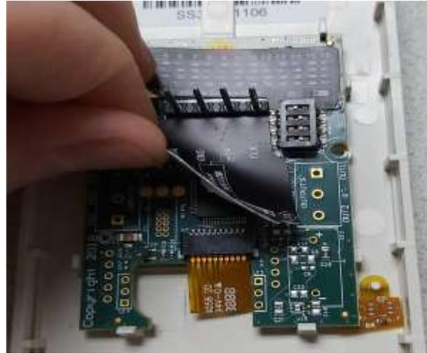
Step # 5: Flex or bend the plastic enclosure in order to release the PCB from the four clips shown.
