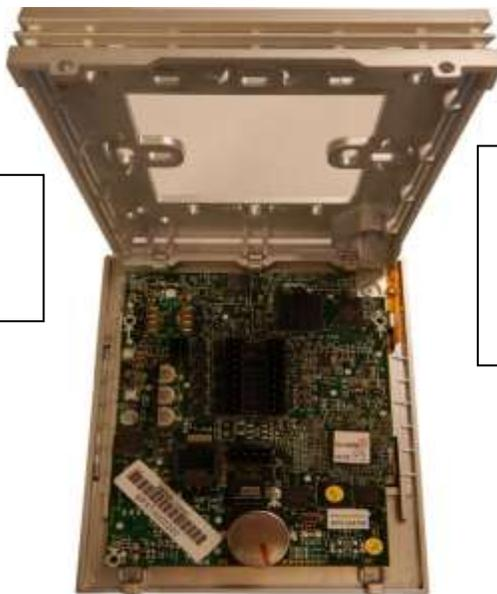
Step # 4: Lift PCB from bottom and disconnect ribbon cables from connectors.
