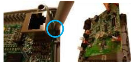
Step # 4: Separate the two PCB's by pulling apart at the connector point.
