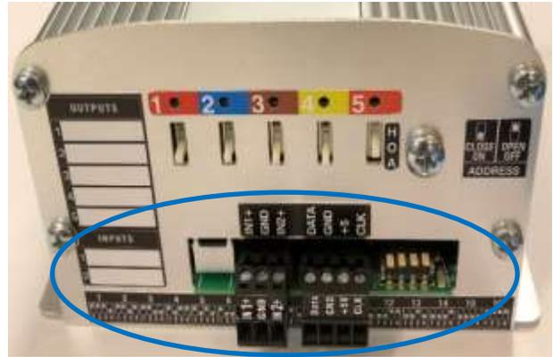
Step # 2: With a Phillips head driver, Remove all 5 Phillips head screws
