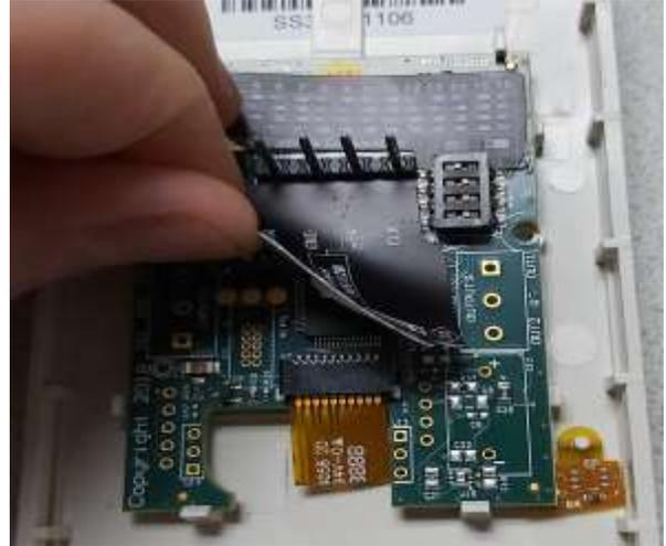
Step # 4: With a Phillips screwdriver, remove two screws from printed circuit board (on applicable options)
