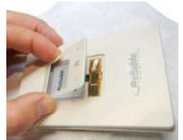
Step # 3: Disconnect flex strip by pulling black tab on connector to release flex strip.
