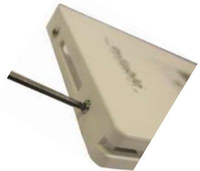
Step # 2: Remove glass by inserting small flathead screwdriver between plastic and glass and gently prying apart to lift up.
