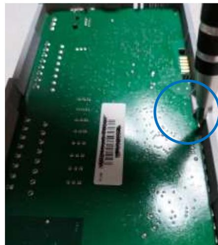
Step # 4: Remove adhesive backed plastic connector label from the circuit board.
