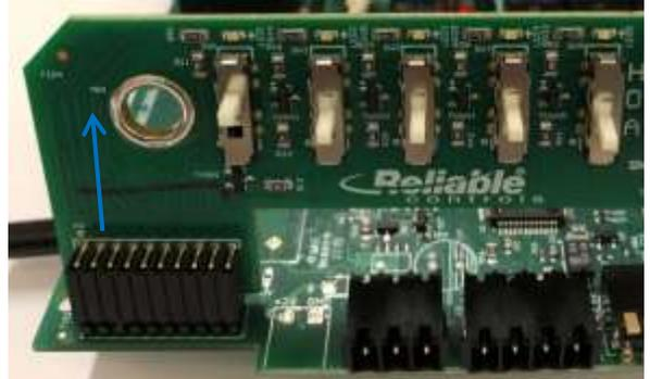
Step # 7: Slide the circuit board away from and out from the aluminum enclosure to discard.
