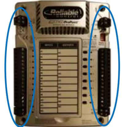
Step # 2: Using small flat head screw driver depress the two plastic tabs on side of controller and pull two sides apart gently.
