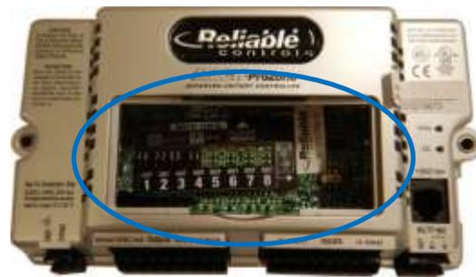
Step # 3: Remove PCB by pulling on plastic tab of enclosure and pushing gently from other side (through top plate opening).
