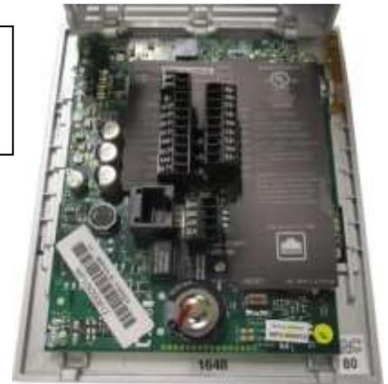
Step # 3: Remove screws holding PCB to plastic housing.
