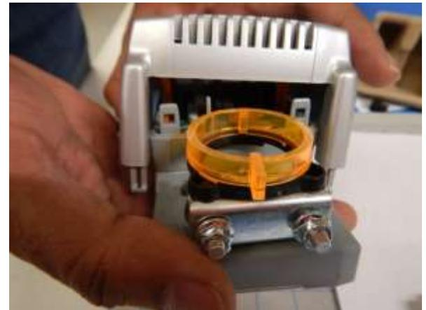
Step # 5: Remove PCB from motor using small flathead screwdriver to depress plastic tab as shown (if applicable).
