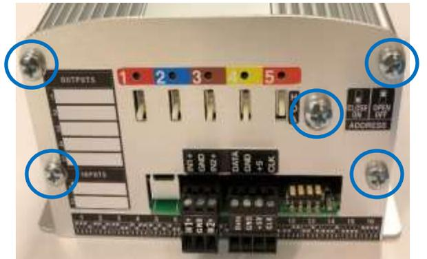
Step # 3: Turn the unit to the other flat side and with a Phillips head driver, Remove 2 Phillips head screws
