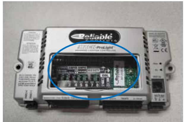
Step # 3: With a small screwdriver, place the slot between the plastic housing and circuit board and push out until the tab releases the circuit board.
