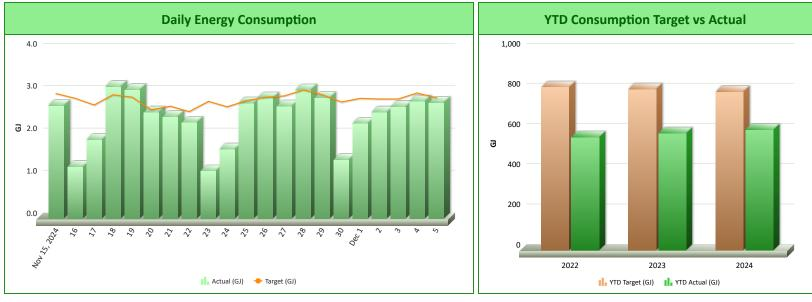
The Reliable Controls BAS calculates a daily energy consumption target in gigajoules (GJ), based on 50% of the ASHRAE standard 90.1 (1999), adjusted for actual heating and cooling degree days. Standard 90.1 is used to predict the energy consumption of an energy efficient building within a specified geographical region. Year to date for 2024, the actual energy consumed by the Reliable Controls South annex remains well below the target.
