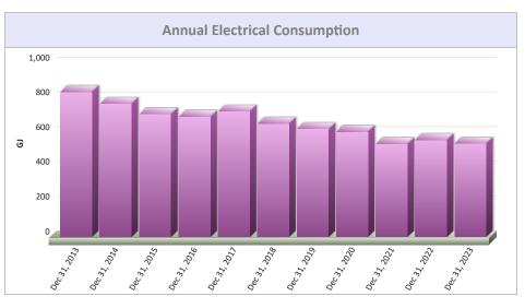
In August 2020, all of the existing T5 flourescent fixtures in the South annex were retrofitted with new LED tubes and drivers. This change led to an instant and ongoing drop in electricity consumption, however, the impact was hidden by occupancy reductions attributable to COVID-19.
